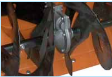
A Robust worm gear for perfect snowblowing !
