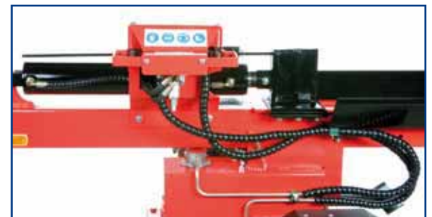
The heart of the log splitter is the hydraulic cylinder in the centre of the machine.
